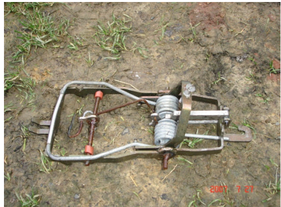
The Set-n-Forget kill trap (a cover is required for ground sets). Similar in design to a rodent snap trap. Trap is sprung through interference with the bait hook, releasing a steel jaw that strikes the animal in the head/neck region.
