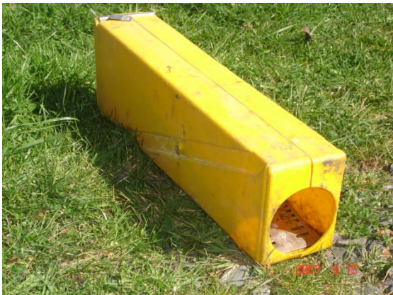
The Holden live capture trap. Bait is placed at the far end of the trap as an attractant and animals are caught when the treadle pivots and locks into place.
