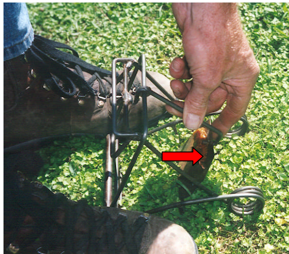
Push trigger plate hole onto the U-shaped end of the trigger plate
