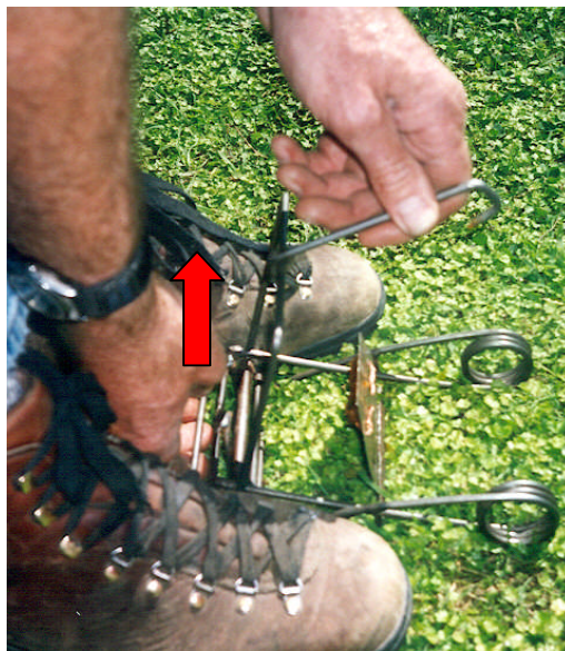
Place feet on bottom bracket and lift striking bar up and hook onto the trigger bar hook.
