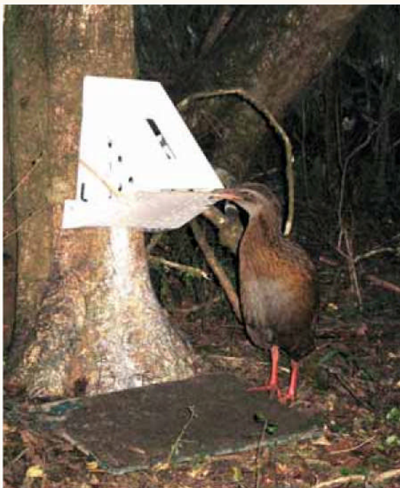
c A wild weka investigates a Sentinel trap fitted with an excluder set over a mud tracking-tray
