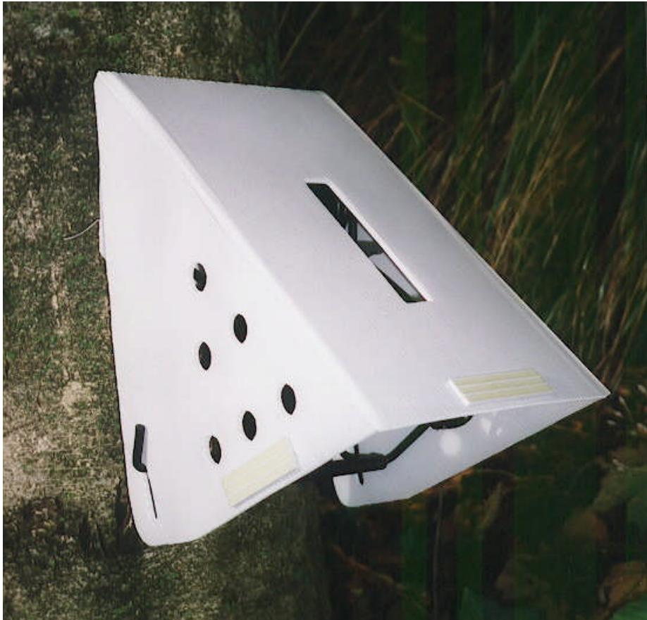
Fig. 6 Attachment of luminescent lures to the sides and top of a Sentinel Kill Trap cover.
