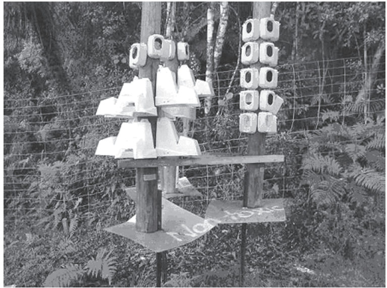
Fig. 1 Bait stations containing gel baits and pellet baits mounted on “possum-proof” poles in the “shaded” bait-weathering enclosure.
